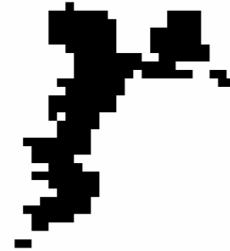
Figure 7. Water body map separated of AVHRR-GAC image and generated by using maximum likelihood classification method
