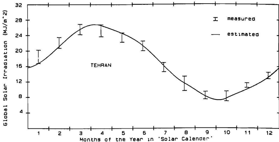
Fig. 1. Comparison of the estimated with measured monthly-mean daily global irradiation on a horizontal surface for Tehran.
