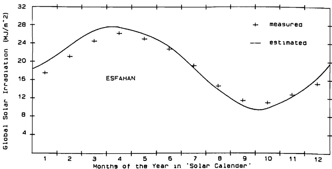
Fig. 2. Comparison of the estimated with measured monthly-mean daily global irradiation on a horizontal surface for Isfahan.
