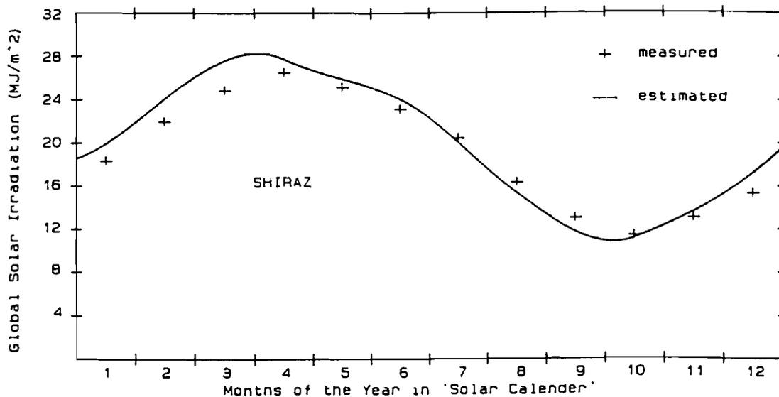
Fig. 3. Comparison of the estimated with measured monthly-mean daily global irradiation on a horizontal surface for Shiraz.
