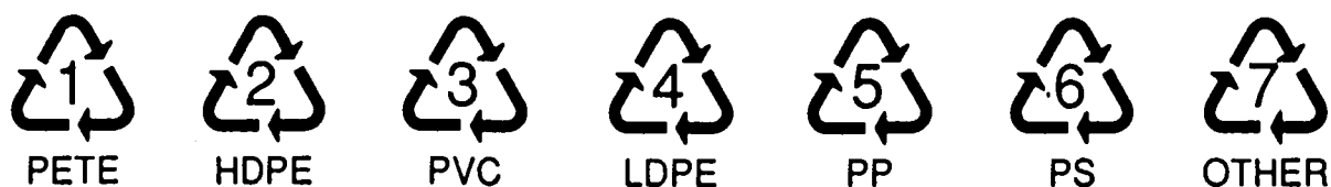
FIGURE 3-1 Code designation used for various types of plastics.
