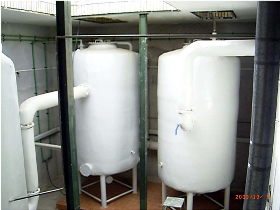
Fig. 2. Anaerobic metallic digestion reactor with 10 m 3 volume used in biogas assessment test.
