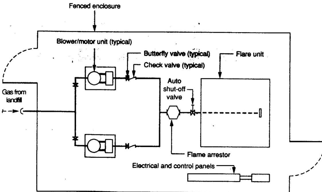
**FIGURE 11-27** Schematic layout of blower/flare station for the flaring of landfill gas. (Courtesy of California Integrated Waste Management Board.)
