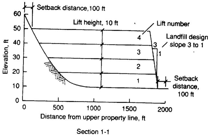
**FIGURE 11-65** Layout of typical landfill for the purpose of estimating the volumetric capacity of a proposed site taking into account setback distances (100 ft), finished landfill slopes (3 to 1), and lift height (10 ft).
