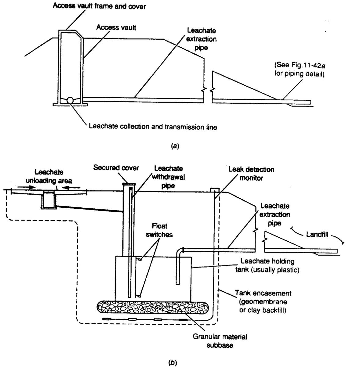
**FIGURE 11-43** Examples of leachate collection facilities: (a) leachate collection and transmission vault and (b) leachate holding tank.
