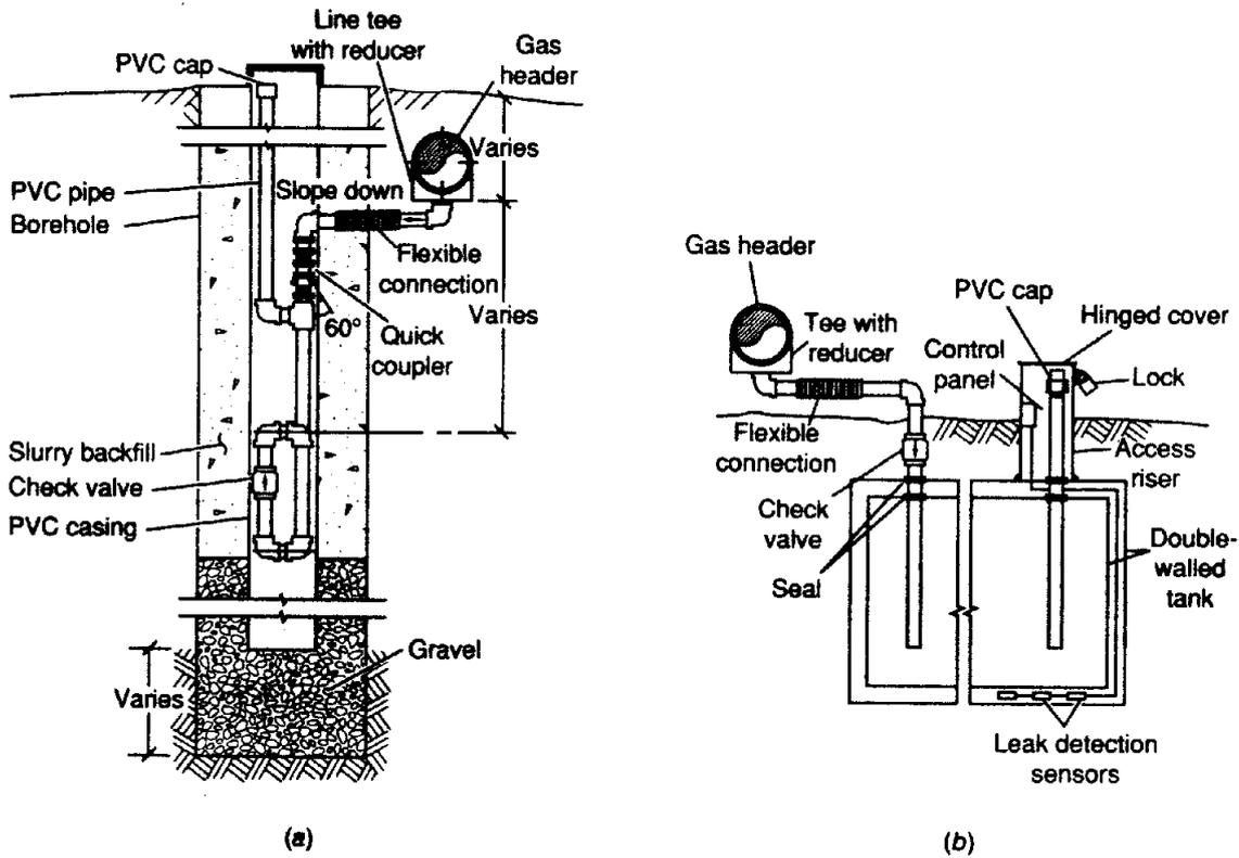
**FIGURE 11-26** Typical condensate traps: (a) liquid is returned to landfill (courtesy of California Integrated Waste Management Board) and (b) liquid is stored in holding tank.
