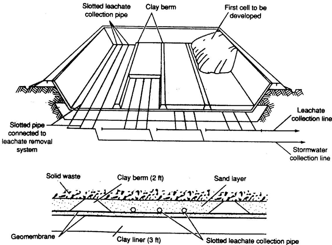
**FIGURE 11-40** Typical leachate collection system using multiple leachate collection pipes: (a) pictorial view and (b) detail of typical leachate collection pipes (adapted from Ref. 33).
