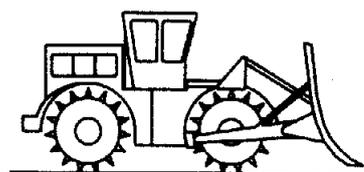
Steel-wheeled compactor with trash blade
