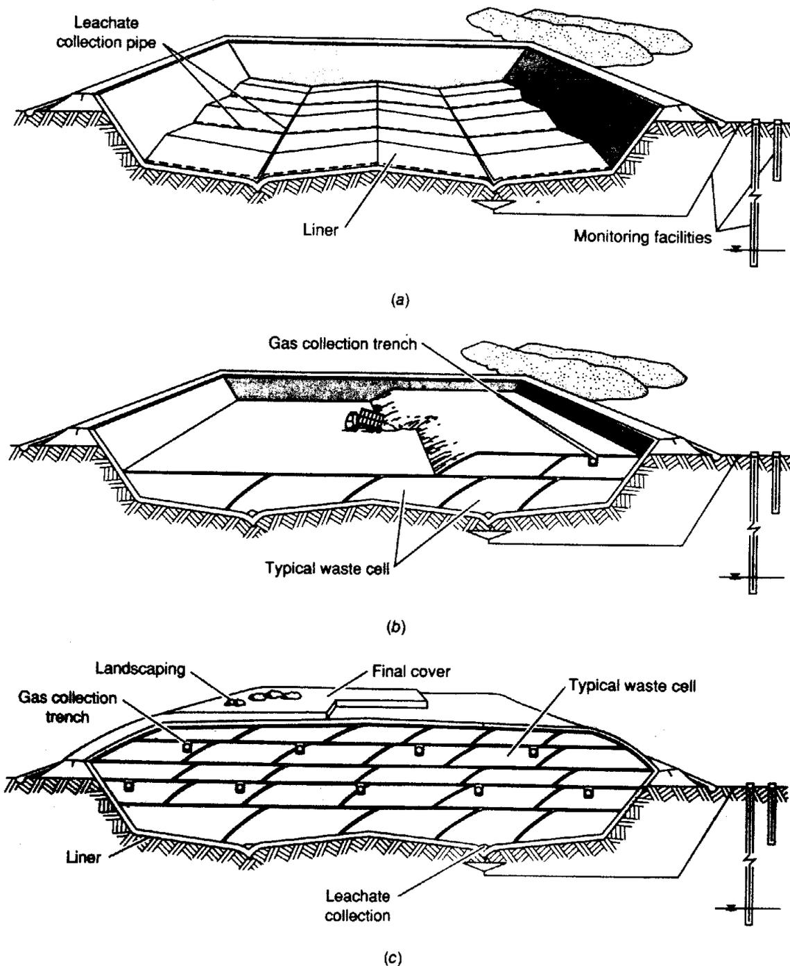
**FIGURE 11-4** Development and completion of a solid waste landfill: (a) excavation and installation of landfill liner, (b) placement of solid waste in landfill, and (c) cutaway through completed landfill.
