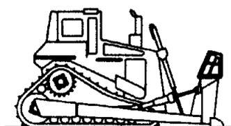
High track compactor with trash blade
