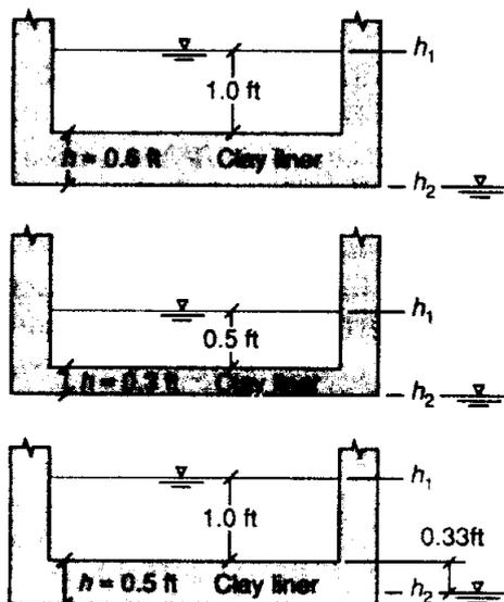
**FIGURE 11-33** Definition sketch for assessing the equivalency of landfill liners. (Note that the discharge through each liner configuration is the same.)
