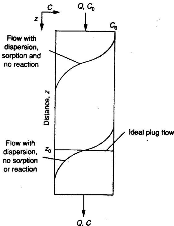
FIGURE 11-35 Typical retardation of trace organic compounds in subsurface movement.
