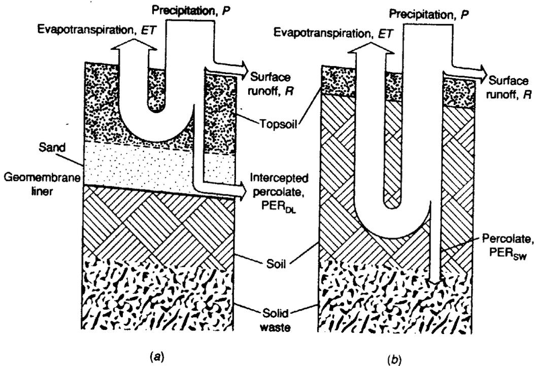
**FIGURE 11-54** Definition sketch for moisture balance for landfill: (a) for landfill cover containing a drainage layer and geomembrane liner and (b) for landfill with no drainage layer (or geomembrane liner).
